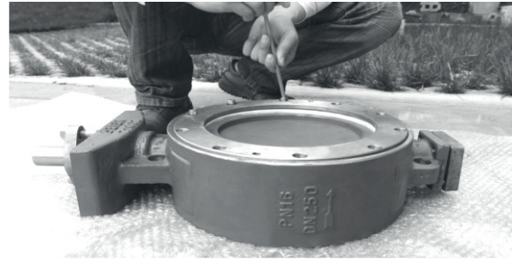
Unload the bolt on insert
