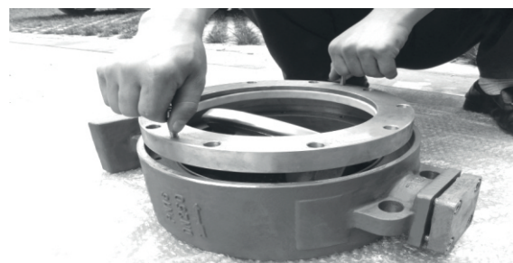
Put the hoop into valve with starting bolt.
