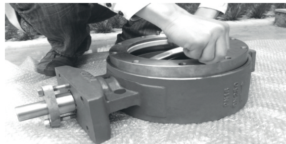
Unload the bolt on insert
